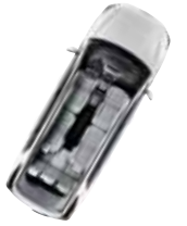
Front and 2 nd -row seats flat (converts into beds for driver and front passenger)
