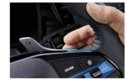
Paddle shifters (Regenerative Braking Control) Paddle shifters add the fun factor by allowing you to control the level of regenerative braking for improved dynamic performance and energy efficiency.
