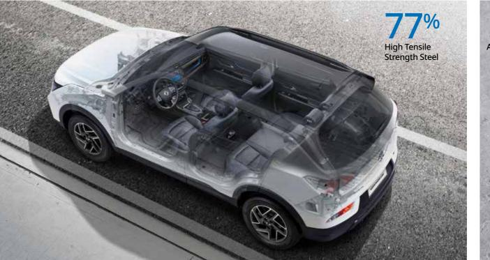
The percentage of high tensile and ultra-high tensile used for the e-Motion's frame has been increased to 77% for increased strength and safety. The passenger safety cell has been structurally reinforced to ensure a higher level of protection in the event of a collision.
